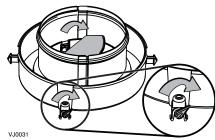
In that case, there is 78 CFM in FRESH air and 61 CFM in EXHAUST air. Then, using the adjusment pin, adjust (close) the FRESH air balancing damper until the FRESH air flow matchs the EXHAUST air flow: 60 CFM (0.2 in. w.g.) with magnehelic gauge connected to FRESH air flow pressure taps).
