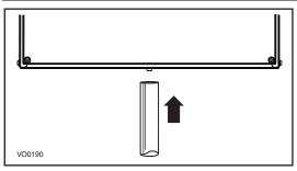
Connect the plastic tube to the inner drain fitting located under the unit as shown.
