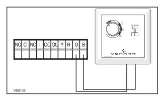
5.4.5 ELECTRICAL CONNECTION TO CONSTRUCTO MAIN WALL CONTROL 5.4.6 ELECTRICAL CONNECTION TO BRONZE MAIN WALL CONTROL (40E, 40H+ AND 50H UNITS ONLY)
