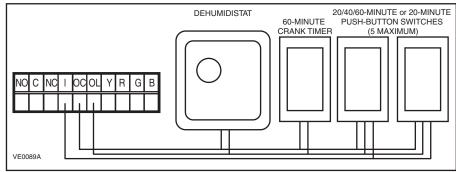
Once the control(s) connections have been made, insert the terminal connector in the electrical compartment interface.
